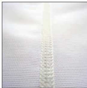
Figure 22 Flat-lock stitch seam is strong, lays flat against the body, and is undetectable under clothing
