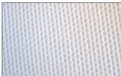
Figure 16 PowerNet fabric consists of a flexible and breathable open hexagon construction
