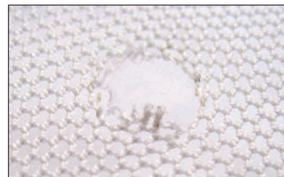
Figure 17 PowerNet resists runs and provides accurate compression even after its structure has been compromised
